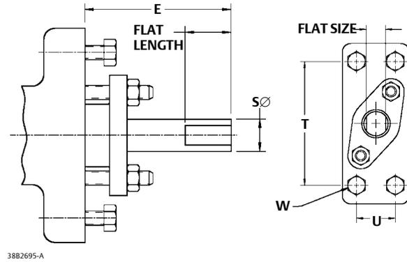
**Figure 4. Fisher V150S NPS 6 Valve**
