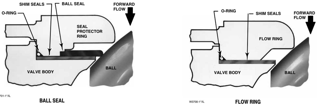
Figure 4. Ball Seal and Flow Ring Constructions
