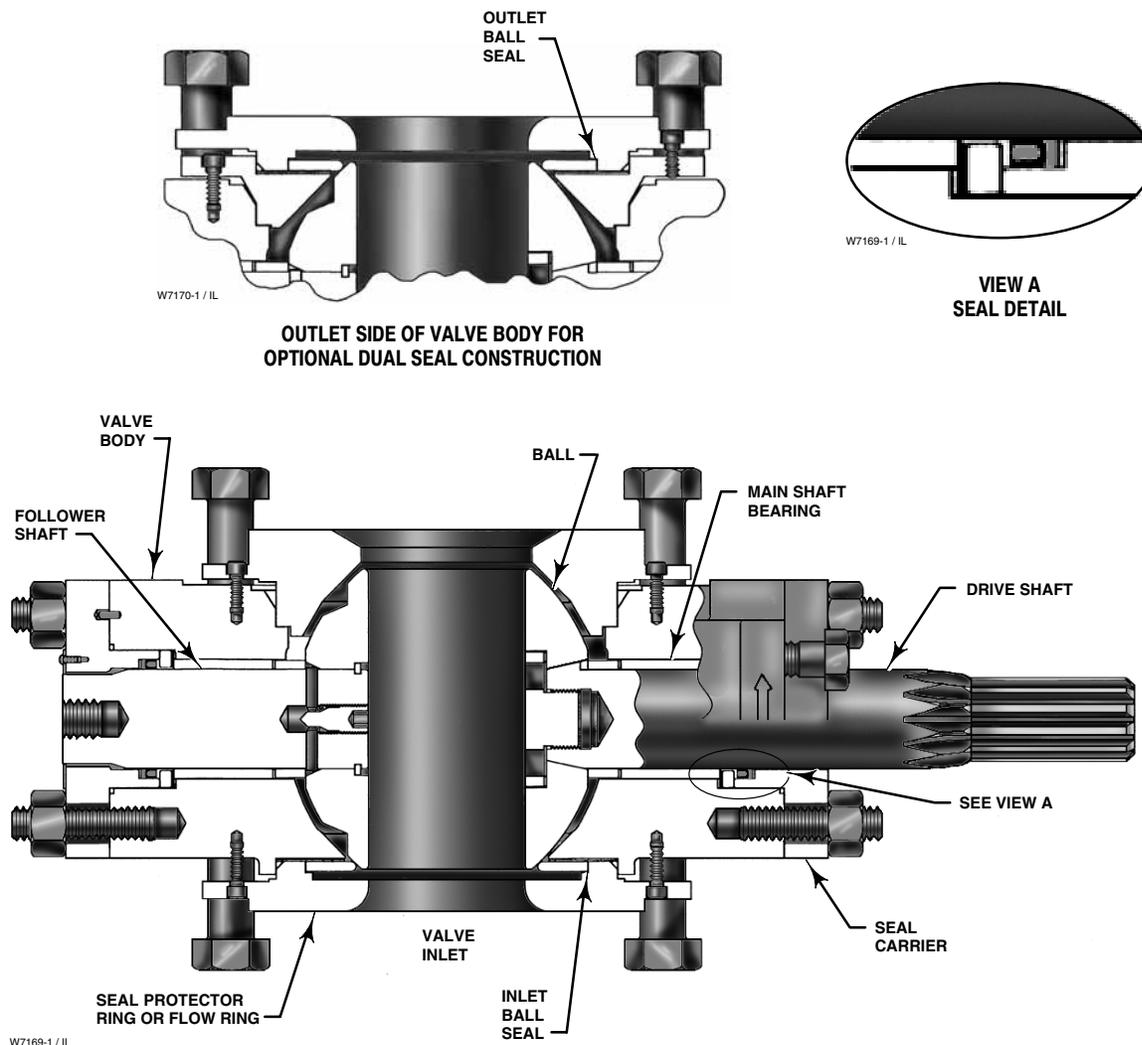
Figure 2. Sectional View of Design V250 Valve
