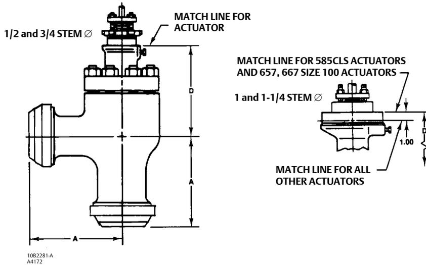
Table 25. NPS 1 through 6 Angle Valve CL2500 Dimensions with Standard Bonnet
