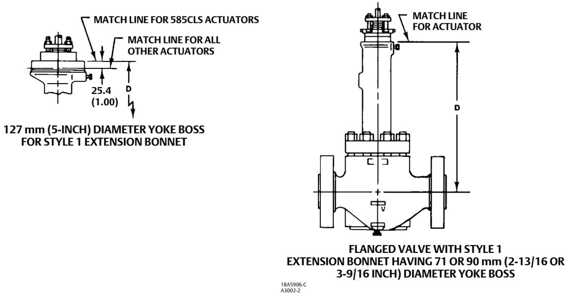
Table 24. Dimension D for Style 1 Extension Bonnet (A, B, and G Dimensions Listed in Figure 23 Do Not Change When Extension Bonnet is Used)
