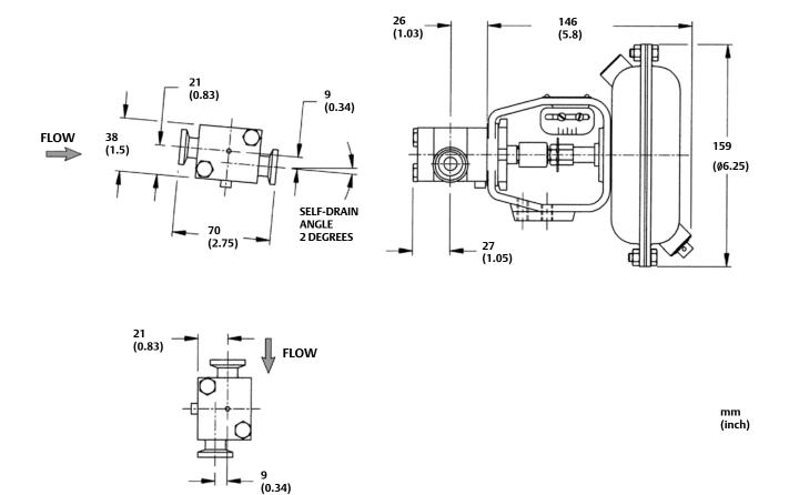
RECOMMENDED MOUNTING FOR SELF-DRAINING (ACTUATOR SHOULD BE MOUNTED HORIZONTALLY)
