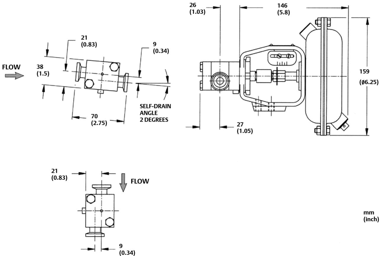
RECOMMENDED MOUNTING FOR SELF-DRAINING (ACTUATOR SHOULD BE MOUNTED HORIZONTALLY)
